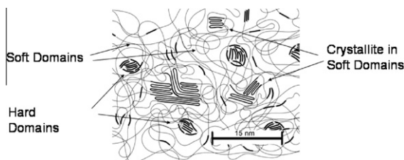
Fig. 12. Schematic representation of SDs crystallization in neat TPU.
